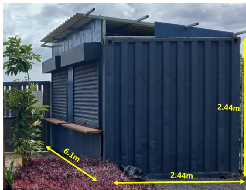
Figure 3: Dimensions of the Commercial Container
